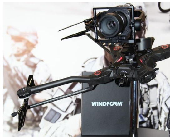
Tundra 3D printed arms in Windform® XT 2.0
