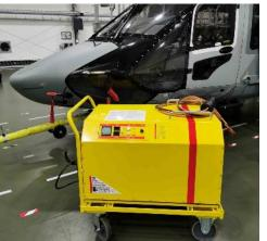
The function: Provide a stabilized external power supply in 28VDC for maintenance or flight preparation and a power capacity to start the engines.
