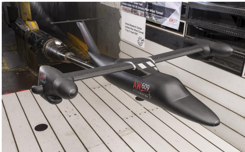
Courtesy of Leonardo HD – Model installed in the 11'x 11' test section at NASA Ames
