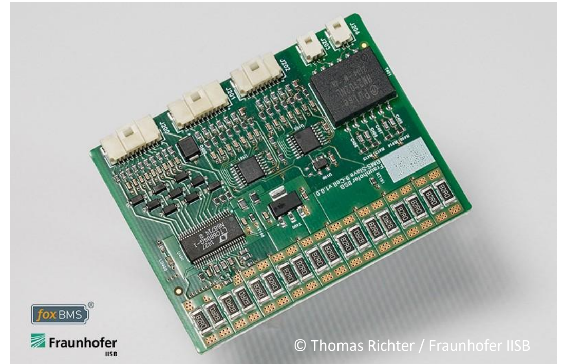
Battery cell voltages and temperatures are monitored by the customized and compact BMS-Slave
