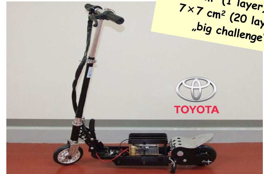
prototype electric kick-board with Solid-state Cells by Toyota
